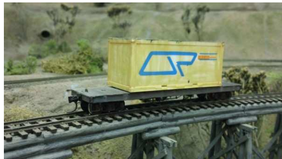
PE wagon (timber) with truss rods
